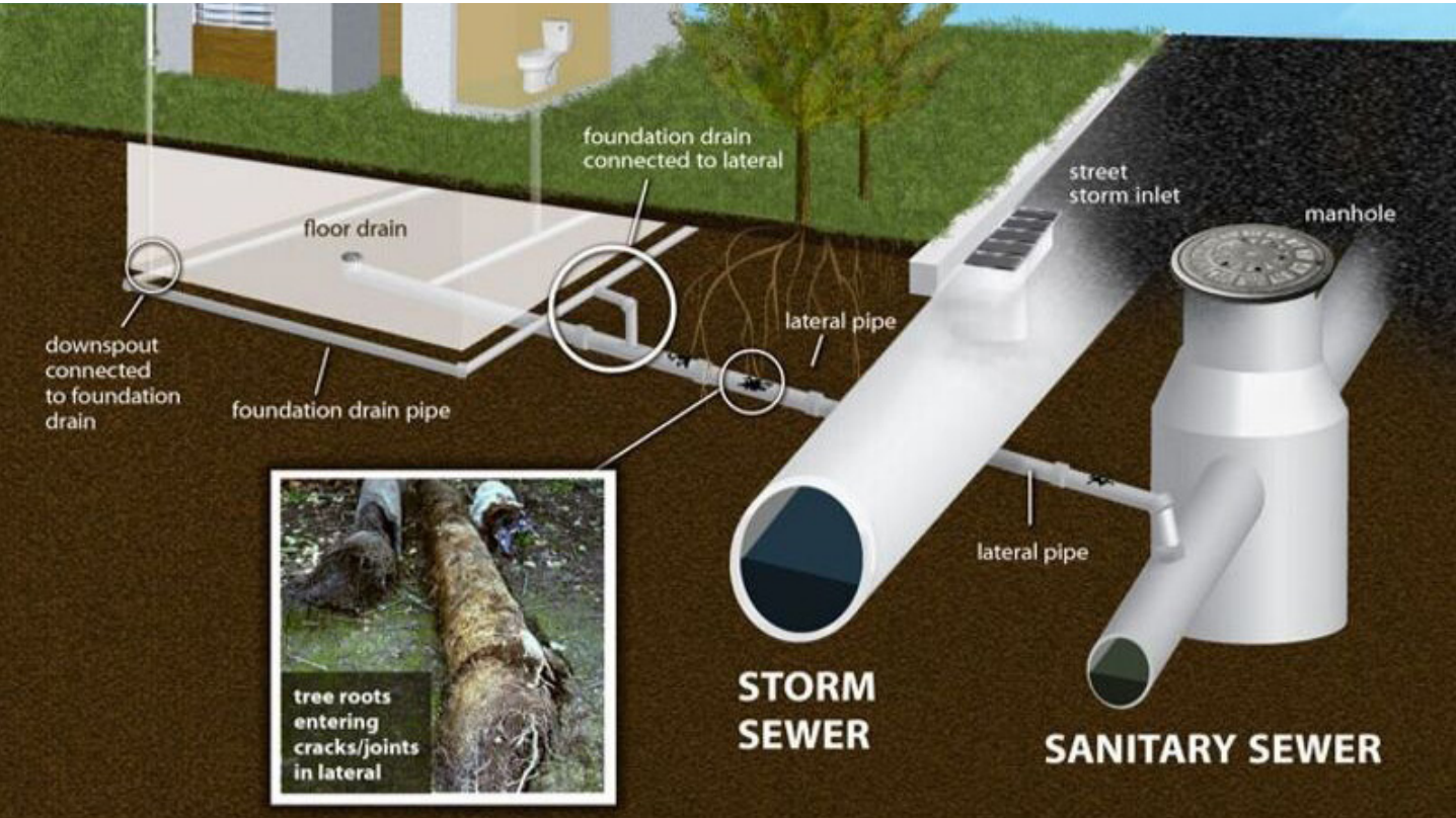
The lateral pipe directs wastewater to the sanitary sewer under the street. Source: MMSD
